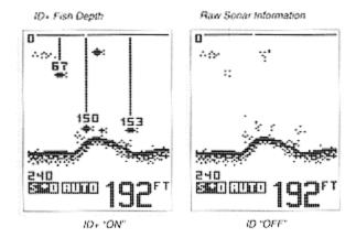
"ID+", the default setting, provides more information about the location of the target by attaching depth "strings" showing the digital depth of the target. When there are numerous targets onscreen, not every target depth is shown, to avoid excessive clutter on-screen.
